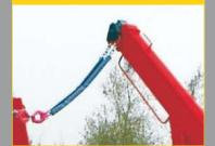
Walk on protection guards, for protection of the piston rod.
