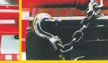
One tipping chain, length 650mm with open safety hook is mounted on the torsion tube. A second tipping chain or tipping hooks are available as an option.
